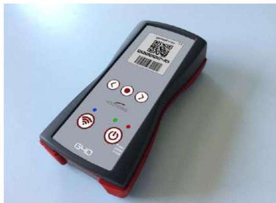
The **G40** unit is a device for control in gas, oil and water distribution and transport networks. Designed for the measurement, monitoring and control of cathodic protection parameters in pipelines.
