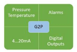
The GOLIAH2P is highly modular device depending on the configuration and the use of the numerous of manageable signals (transmitters, sensors, temperature, digitals). They are available 6 integrated pressure sensors, 2 temperature sensors, 8 digital inputs (for the management of alarms or volume meters), 2 dry contact digital inputs, 8 analogical inputs for transmitters 4-20mA, 2 dry contact digital outputs. The device the PTZ SGERG88 volume correction algorithm.
